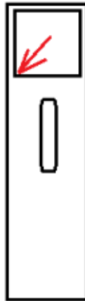
Physical position of the x=0, y=0 pixel on the Minipix (1,1 in Pixet view)
