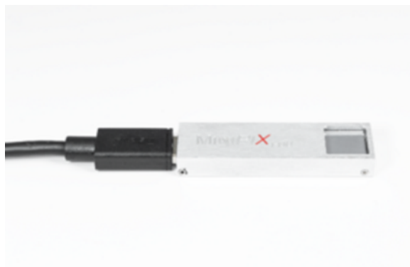
The detector laid flat on the table to collect radiation in a different orientation
