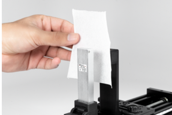
Figure 1. Setup of polonium and camera with tissue paper blocking the path of radiation.
