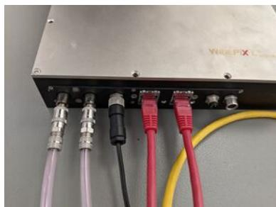
Sometimes it is necessary to synchronize with an external event. Or some instruments, Widepix-L for example, can be organized as set of more than 1 device in 1 box and more than 1 data cable go out. If you want start acquisition on whole instrument at exactly the same time, must use synchronization by the hardware trigger.
